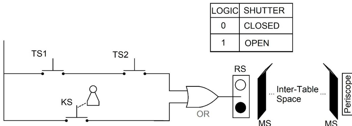
**Figure 2.** Diagram of beam tube interlock logic and beam path blocks.
