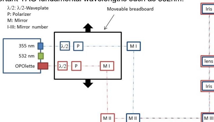
**Figure 1:** Beam path and optical setup for OPOlette use.
