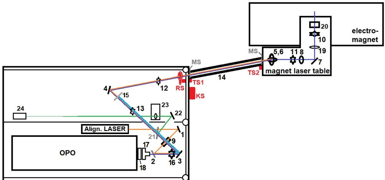
**Figure 1.** Diagram of freespace beam path from GWU-OPO to electromagnet in ICL room F12. The alignment laser might be class IIIIR with safety glasses required. For the local HeNe source, standard amber glasses (LG6) reduce the power to class 2 (500 uW).
