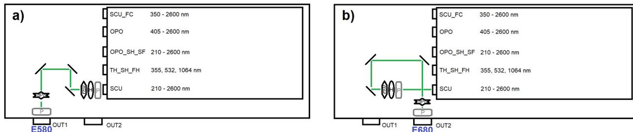
**Figure.** Diagram of freespace beam paths of the Ekspla NT230 for E580 (OUT1) and E680 (OUT2) spectrometers. Panel a) shows the OUT1 path, applicable to the SCU and FH\_SH\_TH outputs. Panel b) shows the scheme applicable to OUT2 path, except SCU\_FC, for going to the E680. Panel c) shows a reconfiguration of mirrors, applicable to OPO and OPO\_SH\_SF. Panel d) shows the optional replacement of the beam splitter (□) with a dichroic mirror (↙).
